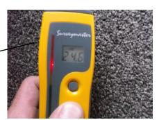
Moisture accumulations here indicate collected water in the door sill channel is 'wicking' past unsealed mitred joinery.
