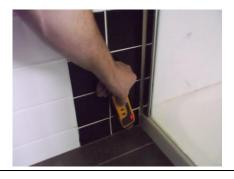
3. In the W corner bedroom W corner exposed timber framing – 41.4% WME and Capacitance mode
